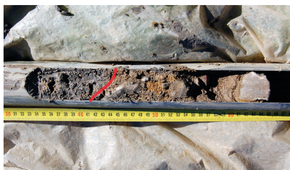
Figure 21. Contact between the bottom of the Holocene permanently submerged facies (to the left) and the Pleistocene gravels (to the right) at 10 m deep in borehole CAR 21
