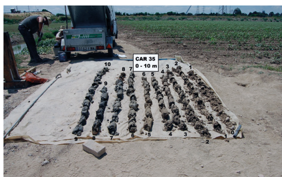
Figure 22. Samples from borehole CAR 35 (0 - 10 m deep)
