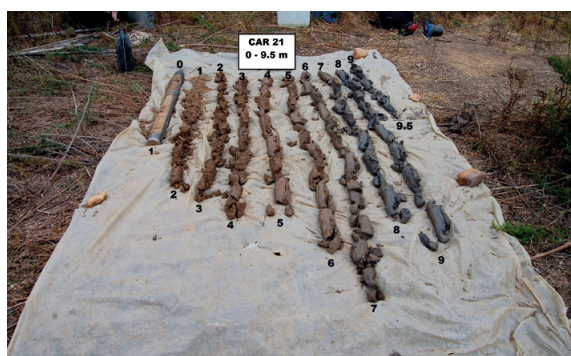
Figure 20. Samples from borehole CAR 21 (0 - 9.5 m deep)
